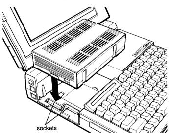
The connectors on the hard disk drive fit into the sockets on the computer.
